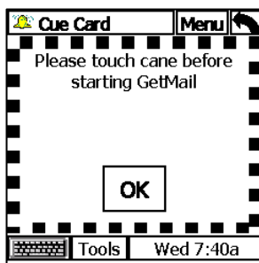
Figure 9: CARE detects that user steps outside without the cane and generates a contingent cue.
