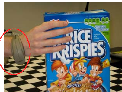
Figure 6: RFID Bracelet detects RFID tag on box
