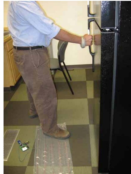
Figure 7: Pressure mat on floor and RFID reader bracelet send wireless data to mobile phone indicating the user is standing in front of the refrigerator and touching the door handle
